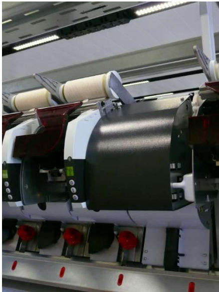
The new VTC installed in the Autocoro 9.
